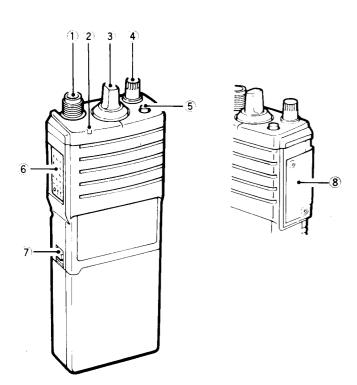
1 ANTENNA CONNECTOR Connects the supplied flexible antenna.
